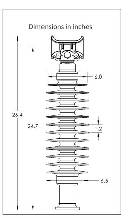
NOTES: [1] Wet-process porcelain insulators are proof tested at 40% of Rated Cantilever Strength [2] MDCL is specified by the manufacturer
