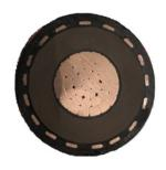
Single conductor power cables allow for ease of splices and terminations which is why Kerite focuses on single conductor solution. In addition to Kerite's unique Permashield® and DR-EPR insulation system, our single conductor PILC replacement design consists of a compact strand that provides up to a ten percent reduction in conductor diameter over full round conductors, flat strap concentric neutrals providing a smaller profile and a polypropylene jacket for additional abrasion resistance.
