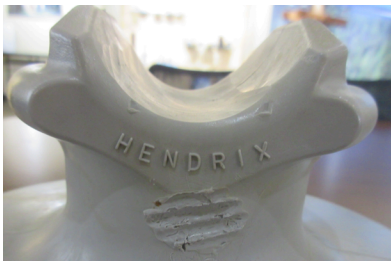
HT Insulator Maximum indent < 1/8" 8hrs: 150C conductor, 150 lb. load.
