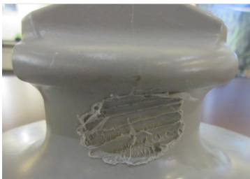
Standard Insulator Maximum indent < 1/8" 2 min.; 150C conductor, 150 lb. load.
