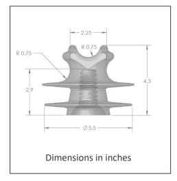
[1] Other pin-hole diameters and thread configurations are available
