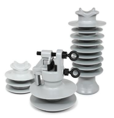
for use with insulated conductors due to the difference in dielectric constants between the porcelain and the polyethylene cable insulation. This incompatibility resulted in the electrical degradation of the cable's jacketing over time. The new polyethylene insulators were compatible with jacketed conductors and caused no damage or erosion to the coating.
