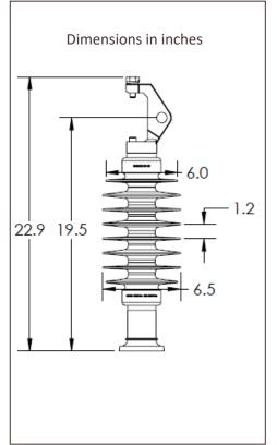
NOTES: [1] Wet-process porcelain insulators are proof tested at 40% of Rated Cantilever Strength
