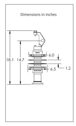
NOTES: [1] Wet-process porcelain insulators are proof tested at 40% of Rated Cantilever Strength
