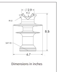
NOTES: [1] Wet-process porcelain insulators are proof tested at 50% of Rated Cantilever Strength
