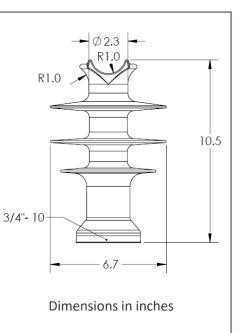
NOTES: [1] Wet-process porcelain insulators are proof tested at 50% of Rated Cantilever Strength
