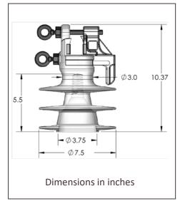
Notes: [1] To specify pin diameter, add the suffix -01 for 1" threads and -02 for 1 3/8" threads (Not available for HPI-15VTP)
