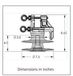
Notes: [1 To specify pin diameter, add the suffix -01 for 1" threads and -02 for 1 3/8" threads
