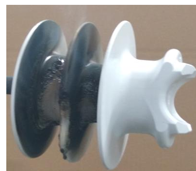
Flame self-extinguished after heat source is removed.
