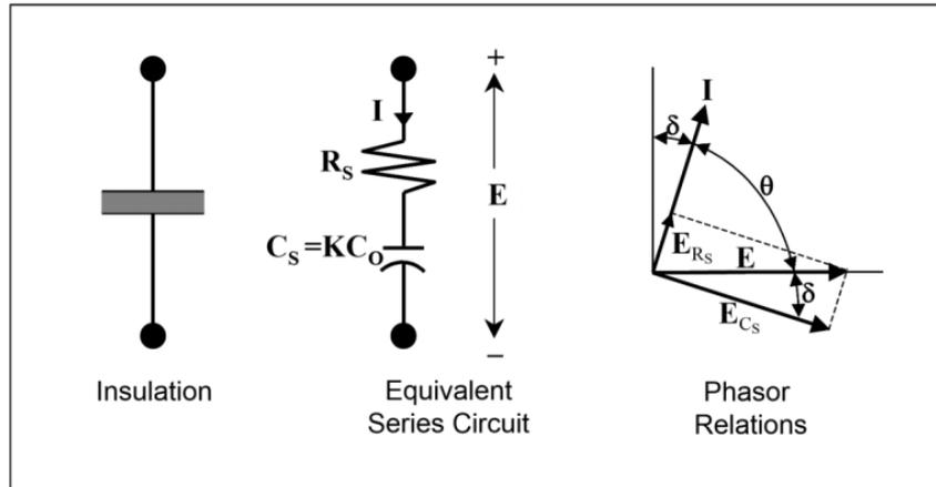
The power consumed (or dissipated) in cable insulation can be reduced to the following relationship in terms of geometry, dielectric constant and dissipation factor.
