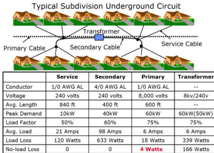
4 Watts with HVK insulation at ambient temperature
