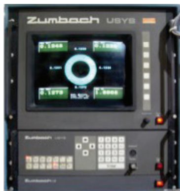
Laser Gauge: Excellent Diameter/Wall Control
